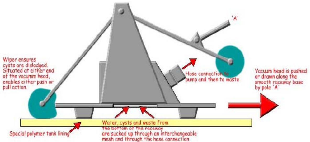
Figure 3.3. The mechanical device or "SystemIch" uses a special suction head connected to a pump that is used to vacuum the bottom of raceways removing the cysts of *I. multifiliis*, faeces and any uneaten food pellets. Trailing wipers ensure that the surface is thoroughly cleaned.
