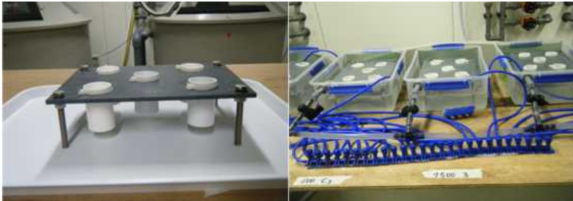
Figure 1: Egg strings were removed from adult female L. salmonis and placed into individual hatching chambers (left) before being exposed to either H 2 O 2 or a seawater control, and placed back into flow through tanks with aeration (right).
